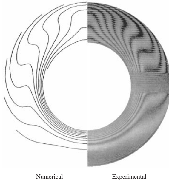
FIGURE 19. Comparison of isotherms at the mid-axial plane for Ra = 1.1 \times 10^4 , R = 2.18 , Pr = 0.7 .
