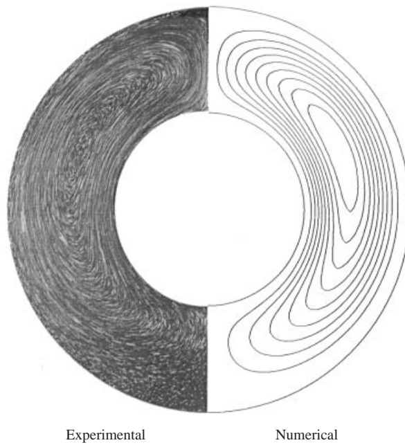
FIGURE 20. Comparison of flow patterns at the mid-axial plane for Ra = 8.725 \times 10^3 , R = 2.1 , Pr = 100 .
